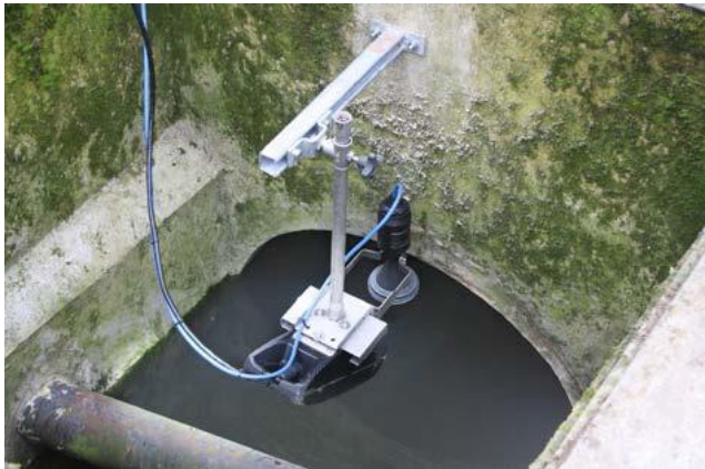
RAVEN-EYE® with radar level sensor
